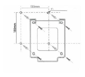
The mounting plate has a hook that the machine will hang onto. Place the machine above it and allow it to slot onto the hook.
