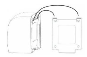
Screw the 'anti-theft' screws into the holes to fix the machine to the mounting plate.
